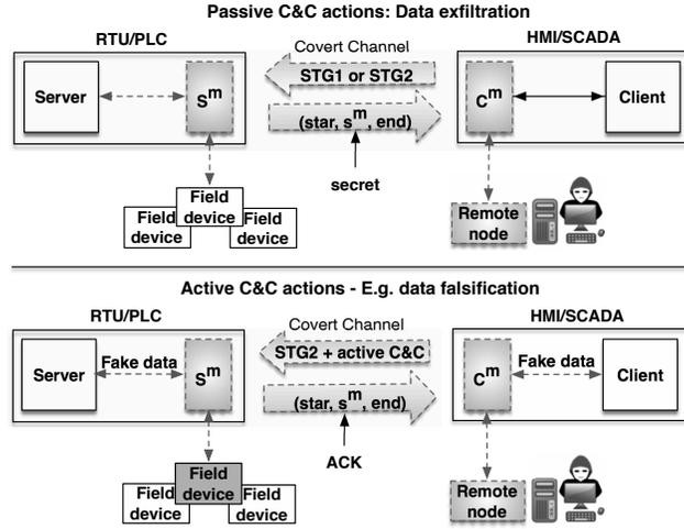
Figure 3: Passive and active actions in OT networks.
