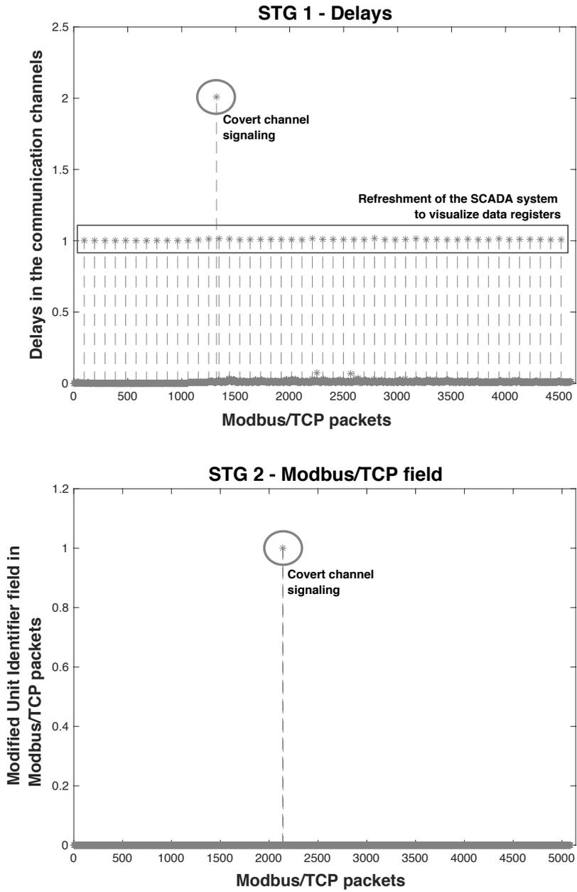
Figure 4: Covert channel using STG-1 and STG-2.
